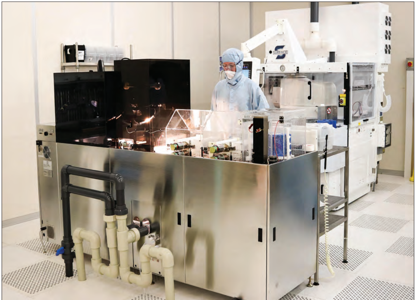
Production of displays involves chemical-mechanical polishing of GaN-on-silicon epiwafers. To reduce the chances of particle contamination, Perspex sheeting is used over the tool.
