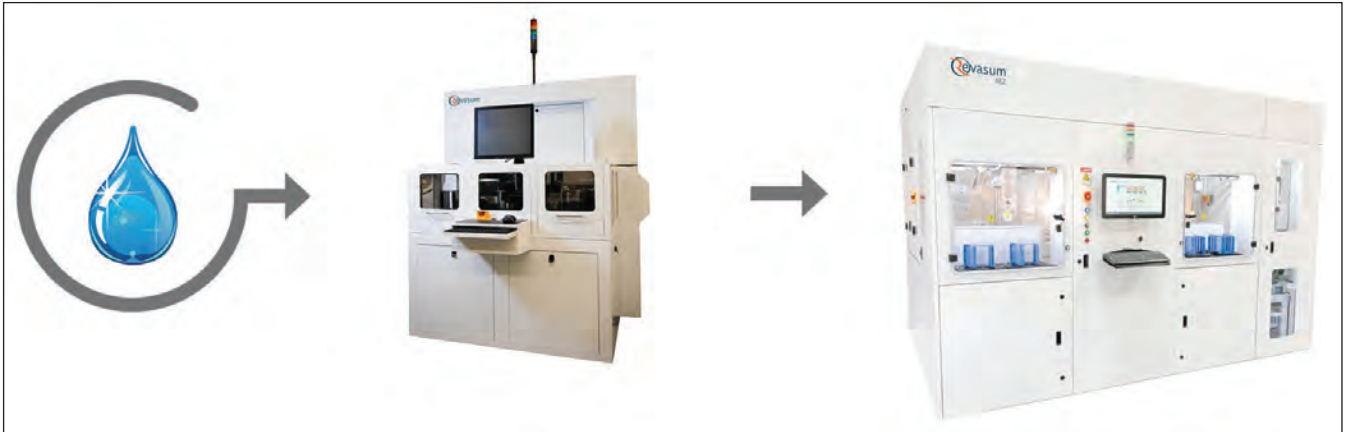
Figure 2. A typical single-wafer processing sequence requires a grinder and a polisher, each with an integrated cleaning module.
