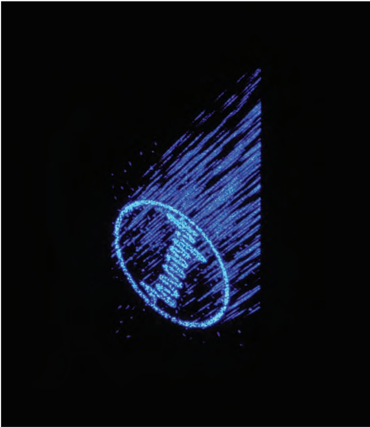
In May 2019, Plessey unveiled a microLED display featuring an array of 1920×1080 current-driven monochrome pixels on a pitch of 8 μm. Each display requires more than two million individual electrical bonds to connect the microLED pixels to the controlling backplane.
